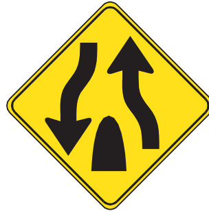
Divided highway ends; two-lane highway begins.
